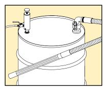
The Dual-Force Vac quickly installs on a UN/1A1/X1.8/300 rated, closed head 55 gallon drum. The drum should be in good condition free of dents or rust.
